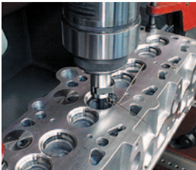
Picture 3 - Cutting valve seat inserts
