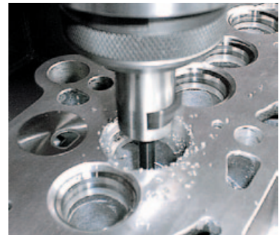
Picture 5 - Cutting the counter bore
